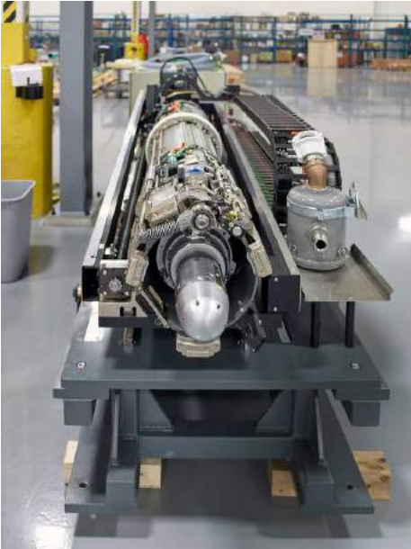
ATS Automation helped develop the bellows cut tool, which will help remove the reactor's fuel channels.
