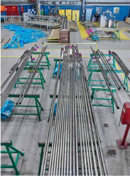
Some of the 7,600-odd feeder pipes BWXT is manufacturing to bring coolant into the reactors.
