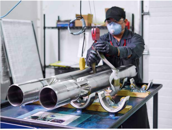
A worker at Toronto's Triumph Gear Systems crafts shield plugs for end fittings.
