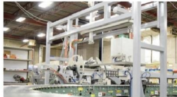
PROMATION's pick-and-place solution incorporates Festo's EXCT-100, a two-axis, high speed linear gantry.
